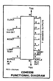
segment display device used for representing the decimal numbers 0 to 9. The 7-segment outputs go high on selection in the CD4033B; in the CD4026B these outputs go high only when the DISPLAY ENABLE IN is high.
