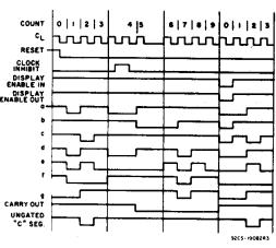
Fig. 3 — CD4026B timing diagram.
