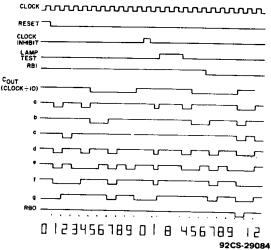
Fig. 4 -- CD4033B timing diagram.
