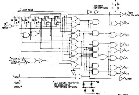
Fig. 2 - CD4033B logic diagram.
