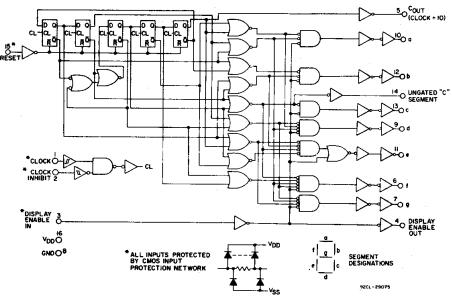
Fig. 1 - CD4026B logic diagram.
